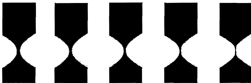
Figure 1: The decay of a liquid bridge of magnetic fluid (APG S11). The time lapse between consecutive pictures is \Delta t = 0.5 ms.
