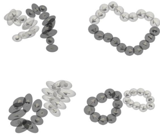
Figure 1: Pair of chains (top line) and rings (bottom line) for spheres and ellipsoids. The distance between middle particles is 3 and square of magnetic moment is 5.
