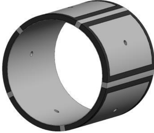
Figure 3: A schematic overview of a hybrid bearing with MR texturing. The bearing works as a MR textured hydrostatic bearing at low speeds and as a conventional HD bearing at high speeds (see Figure 1).
