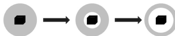
Figure 1: Sketched inside-out etching mechanism of a silica shell (grey) with magnetic core (black).
