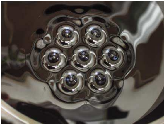
Figure 1 Photo of a localized patch of seven spikes on a layer of ferrofluid.
