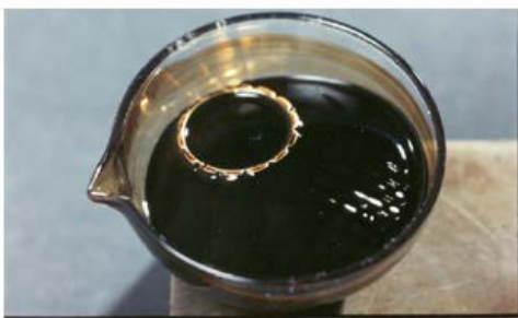
Fig. 1 a suspended golden ring is floating on the surface of a water-based 30mT MF in presence of a Ba-Ferrit permanent magnet.
