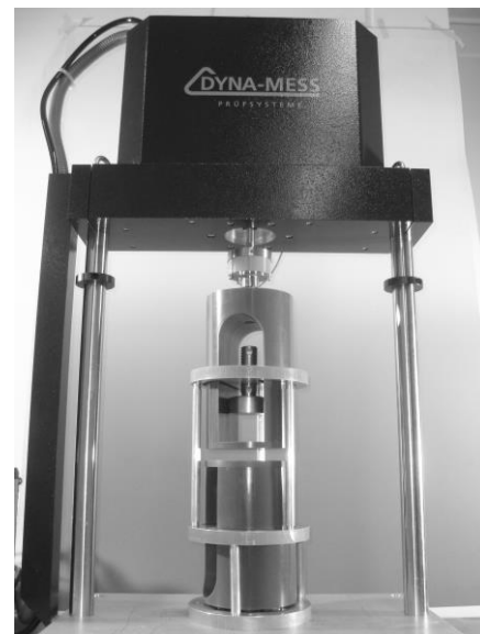
Fig.2: magnetic field dependent stress test
