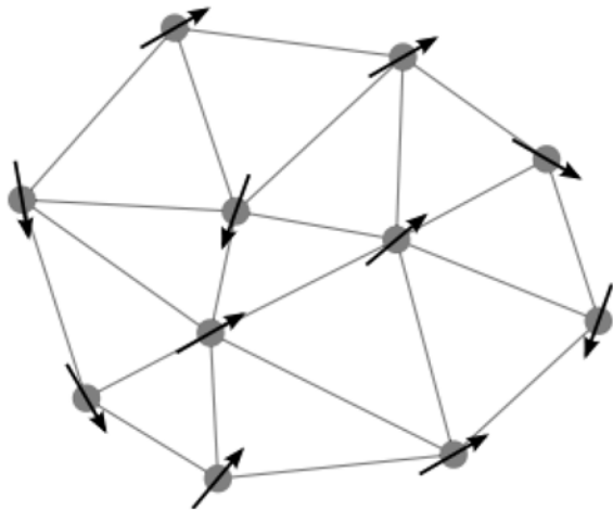
Figure 2: Model sketch for ferrogels without orientational coupling to the elastic matrix.
