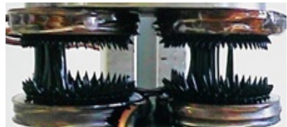
Fig. 2 Picture of a drive engine model: a couple of electro magnets were filled with magnetic fluids to increase the permeability between the pole shoes.
