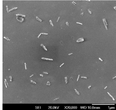
figure 4a: SEM image of nickel nanorods.
