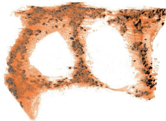
Figure 1: Highly resolved 3D reconstruction, single particles and polyurethane matrix visible.
