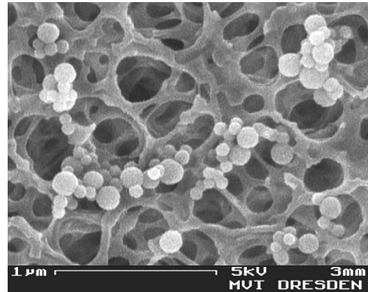
Fig. 1: SEM-image of iron oxide particles synthesized from a 0.3 mmolar iron chloride solution with 5m% ethanol, atomized at 1.7 MHz.
