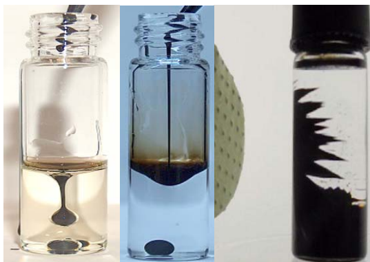
Figure 1. Perfluoropolyether-based Co-MF (a) in hydrocarbon, (b) in water and (c) in silicone oil.
