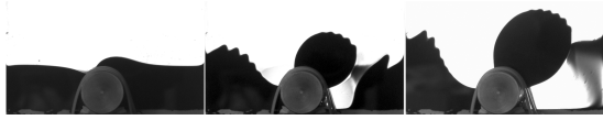
Figure 2: Process of contour deformation in the increasing magnetic field ( 60^\circ inclination), photo series.
