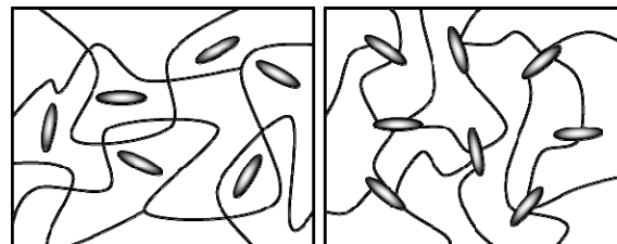
Scheme 1: MBA-crosslinked ferrohydrogel with ellipsoids (left) and ellipsoid crosslinked ferrohydrogel (right).
